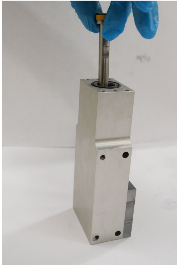
Figure 25: Install Metering Piston
