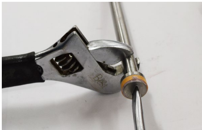
Figure 16: Remove Lip Seal Screw
