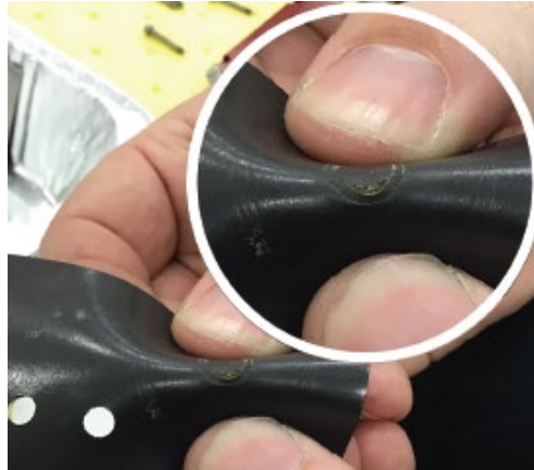
Figure 9: Worn Pump Gasket
