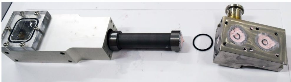
Figure 13: Remove Metering Sleeve from Metering Body
