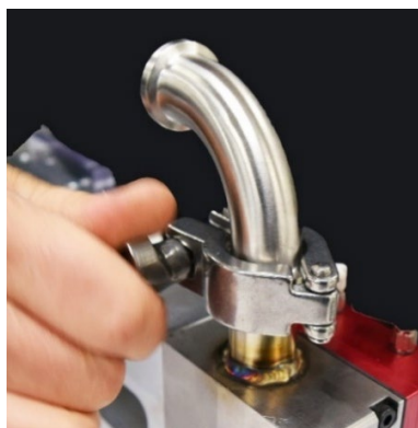
Figure 31: Install the Clamp
