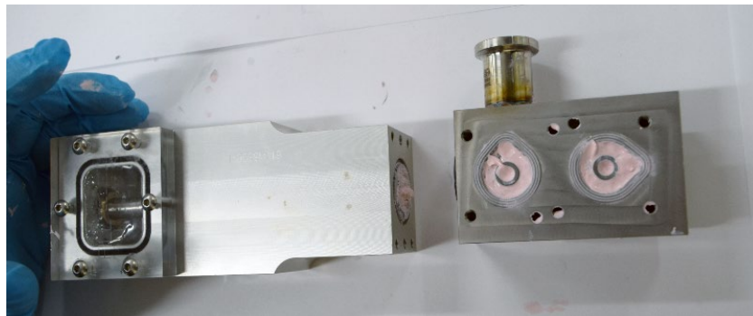
Figure 12: Separate Fluid Distribution Block from Metering Body
