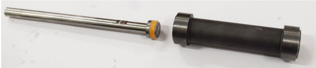
Figure 14: Remove Metering Piston from Metering Sleeve
