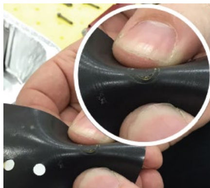
Figure 10: Worn Pump Gasket
