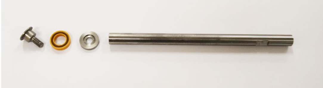
Figure 17: Lip Seal Screw, Teflon Washer, Metering Piston Disassembled
