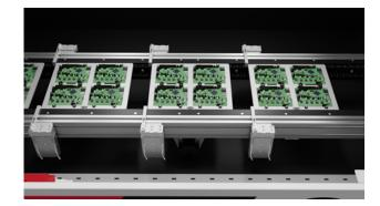
$^{\infty}$  Part handling: Edge chain conveyor with hand crank rail width adjustment, left to right
