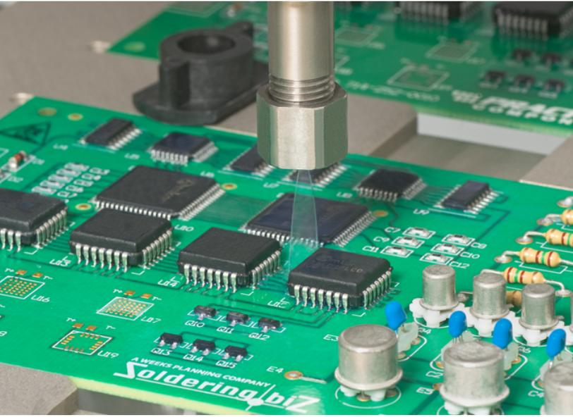
**Conformal coating** is a protective coating or polymer film that “conforms” to the circuit board’s inherent irregularities to protect electronic circuits from harsh environments. Conformal coatings are a breathable protective layer that protects a printed circuit assembly from its exposed environment by filtering out airborne contaminants and maintaining long-term surface insulation resistance. Entrapped moisture, however, is allowed to escape.
