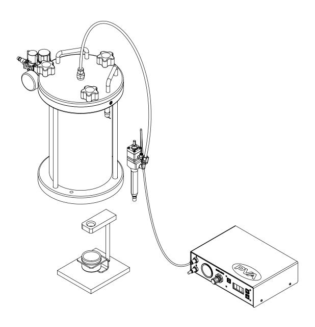
System shown above includes optional PV105-1 Valve Stand with solvent/purge cup.
