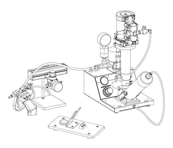
System shown above includes optional PV106-S Valve Stand with solvent/purge cup.
