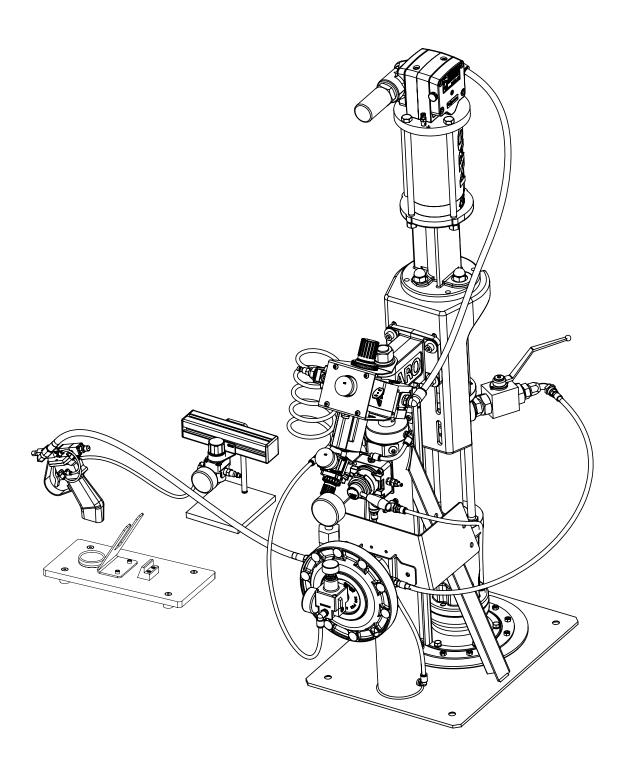
System shown above includes optional PV106-S Valve Stand with solvent/purge cup.
