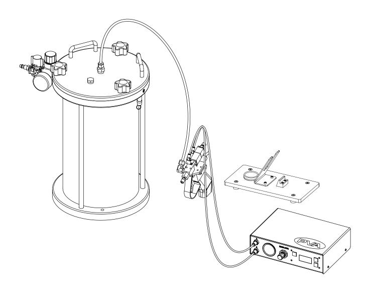
System shown above includes optional PV106-S Valve Stand with solvent/purge cup.
