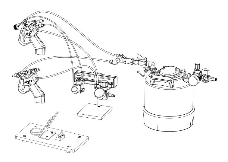
System shown above includes optional PV106-S Valve Stand with solvent/purge cup.
