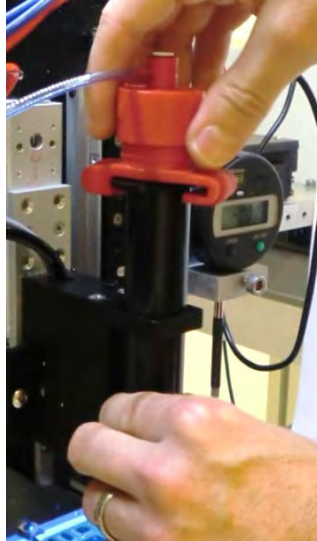
Figure 9: Attach the Air Cap
