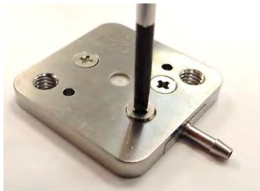
Figure 22: Install the Nozzle Plate Screws
