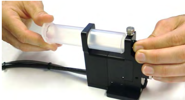
Figure 8: Install the Fluid Syringe
