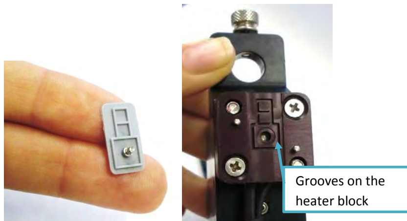
Figure 2: Diaphragm and Heater Block Grooves
