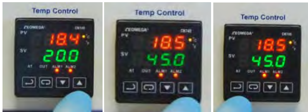
Figure 34: To Change the SV Temperature
