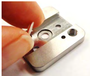
Figure 20: Install the Orifice
