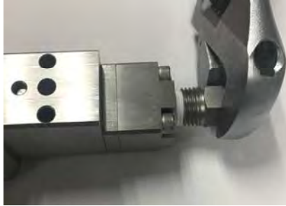
Figure 55: Assemble Luer Adapter
