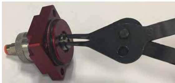
Figure 20: Remove Snap Ring
