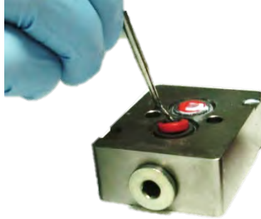
Figure 23: Remove Lip Seals From Fluid Section
