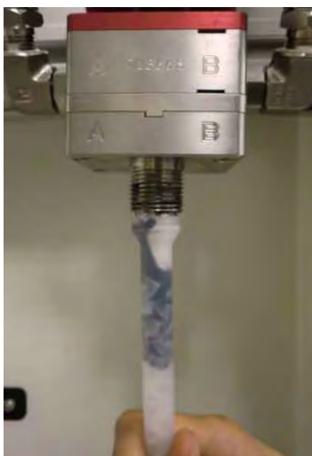
Figure 4: Fill the Static Mixer
