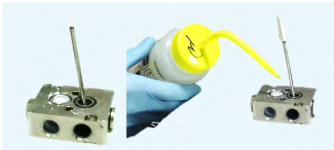
Figure 28: Clean the Fluid Section
