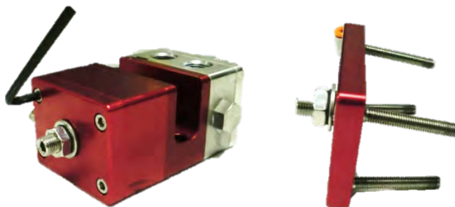
Figure 11: Remove Air Cap Screws
