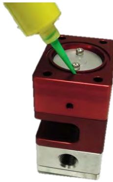
Figure 50: Apply Grease to Air Cylinder Groove
