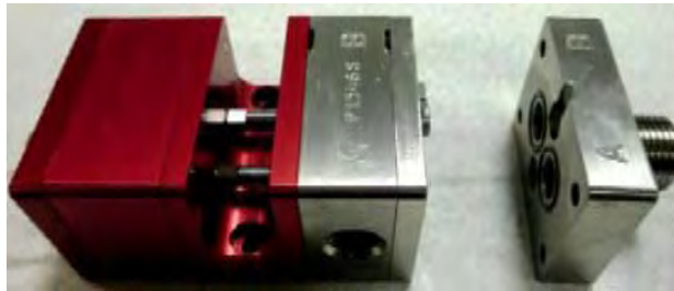
Figure 57: Fluid Manifold Aligned with Valve
