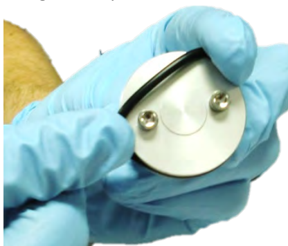
Figure 33: Put the O-ring on the Piston
