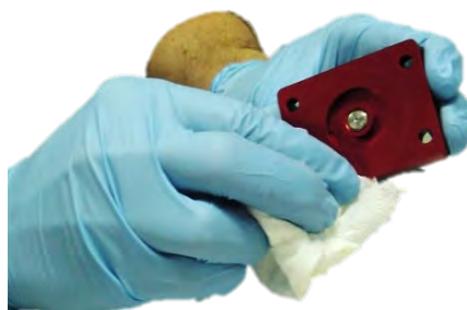
Figure 27: Clean the Cylinder Cap
