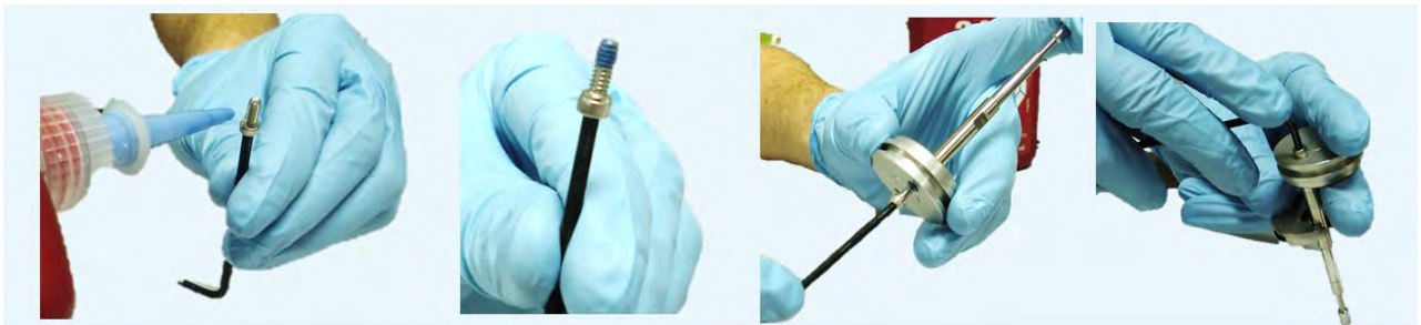
Figure 30: Install Screw in the Piston-Rod Assembly
