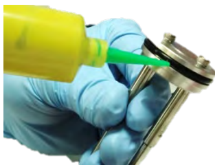
Figure 45: Apply Grease to the O-ring
