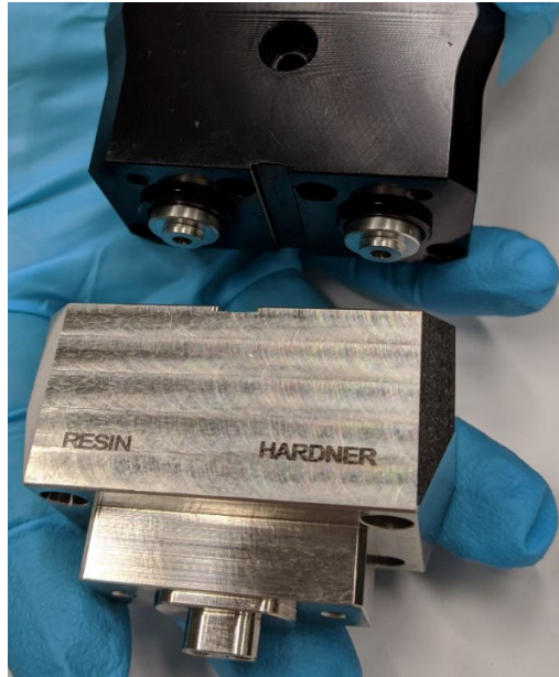
Figure 53: Install Manifold onto Twin Block
