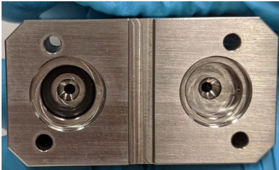
Figure 52: Install O-Ring onto Manifold Block
