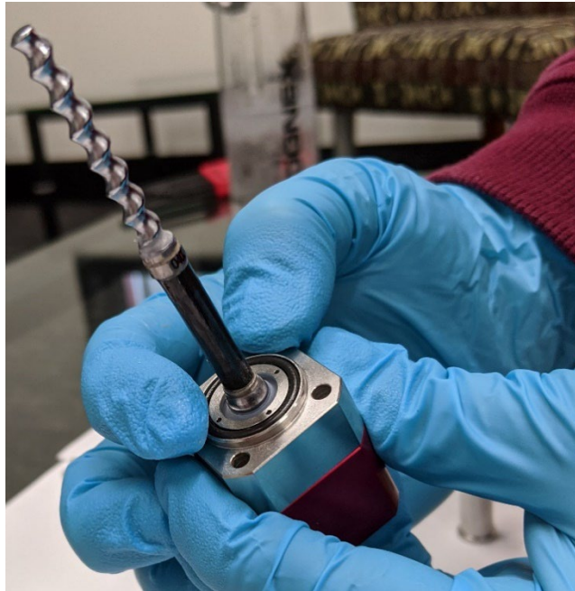
Figure 32: Install O-Ring on Seal Block
