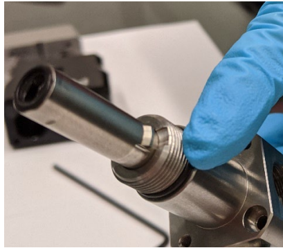
Figure 37: Install O-Ring on Fluid Block Assembly
