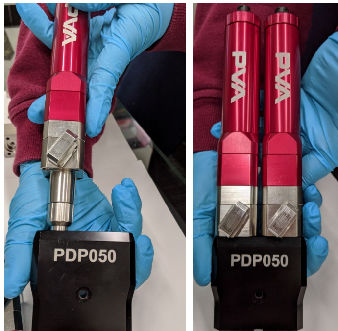
Figure 50: Install Pumps on Twin Block
