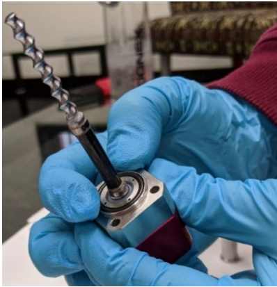
Figure 25: Remove O-Ring from Seal Block
