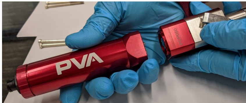
Figure 14: Separate Motor from Rotor Assembly
