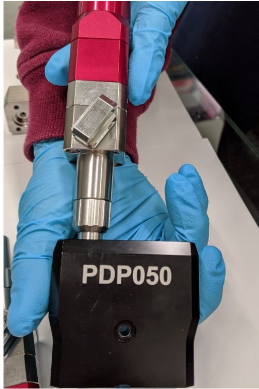
Figure 13: Remove Pumps from Twin Block
