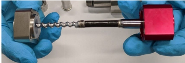
Figure 29: Install Seal Block on Rotor Assembly
