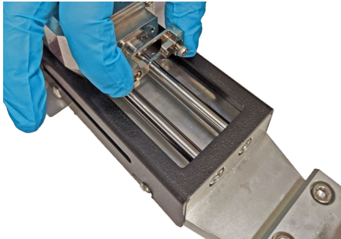
Figure 5: Remove Static Mixer Collar and Screws
