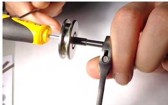
Figure 27: Disassemble the Piston-Rod Assembly
