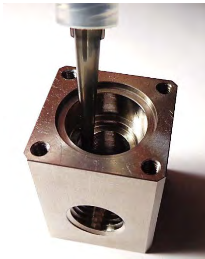
Figure 56: Apply Lubricant to the Fluid Body
