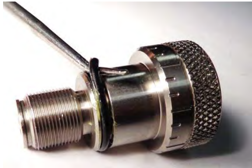
Figure 31: Remove the O-ring from the Stroke Adjust
