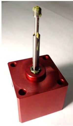
Figure 53: Rod O-ring Installed
