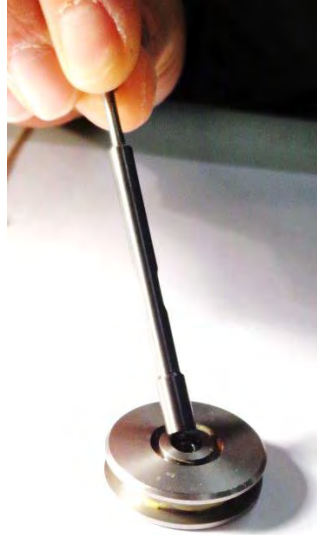
Figure 49: Rod on the Grooved Side of the Piston
