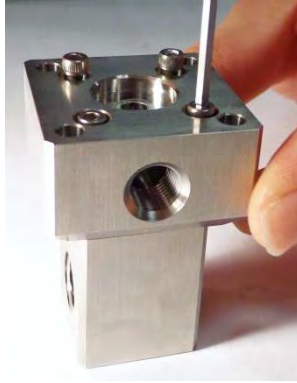
Figure 60: Tighten the Separation Body Screws
