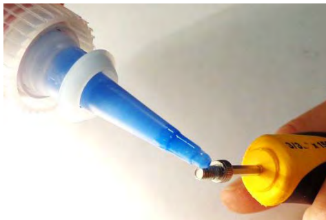
Figure 48: Apply Removable Thread Locker
