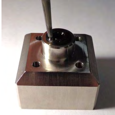
Figure 55: Apply Lubricant to the Top of the Lip Seal
