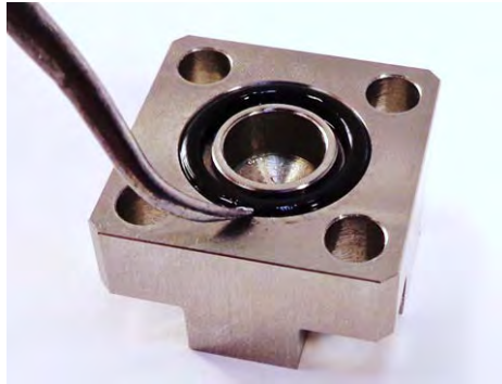
Figure 17: Remove the O-ring from the End Cap
