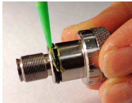
Figure 42: Apply Grease to the O-ring
