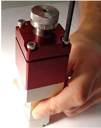
Figure 77: Tighten the Air Cap Screws
