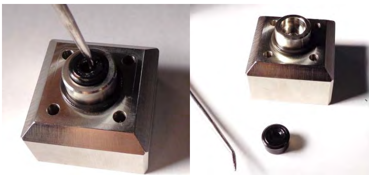
Figure 8: Remove the Lip Seal
