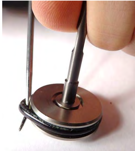
Figure 26: Remove the Piston O-ring
