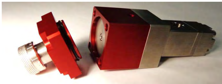
Figure 75: Install the Air Cap
