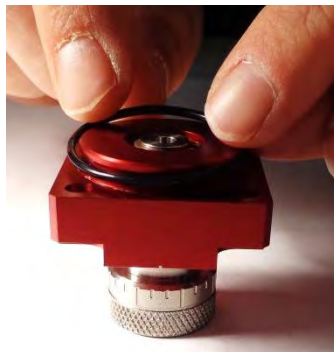
Figure 45: Install the Air Cap O-ring
