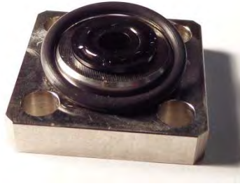
Figure 63: Install the Seal Plate O-ring
