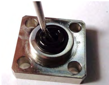
Figure 20: Remove the Lip Seal
