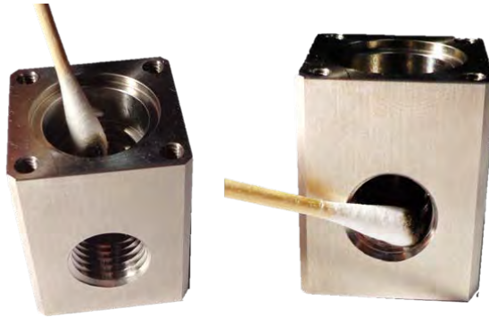
Figure 35: Clean the Fluid Body
