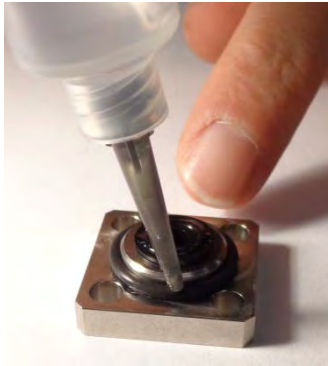
Figure 64: Apply Lubricant to the Seal Plate O-ring
