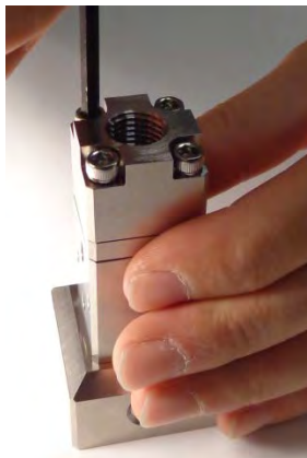
Figure 70: Tighten the End Cap Screws Equally
