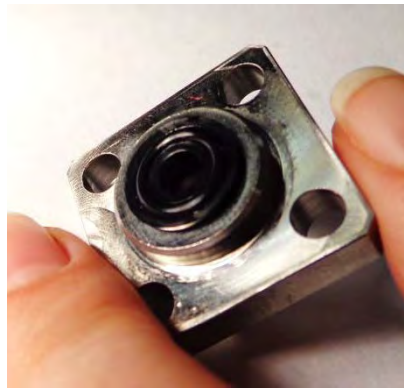
Figure 61: Lip Seal Install O-ring Up
