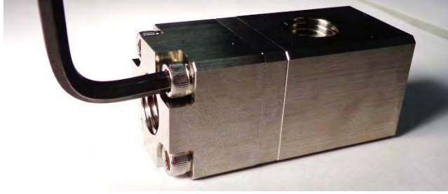
Figure 10: Remove End Cap Screws
