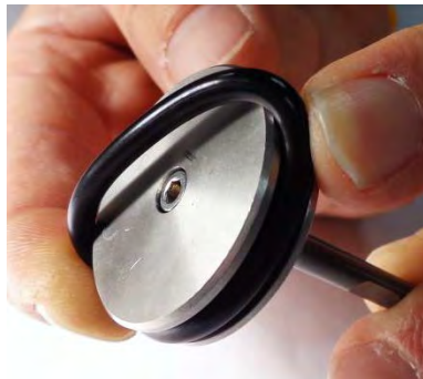
Figure 51: Install the Piston O-ring
