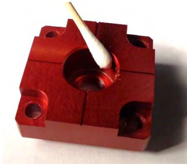
Figure 38: Clean the Air Cap
