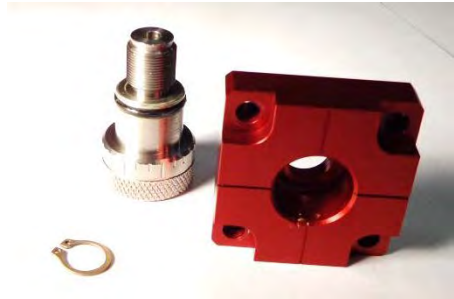
Figure 30: Stroke Adjust Removed from Air Cap
