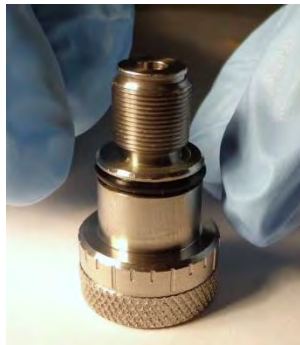
Figure 39: Install the Stroke Adjust O-ring
