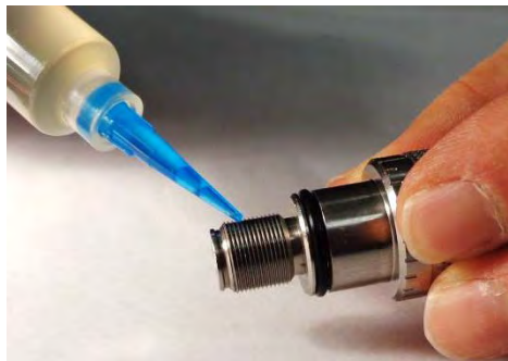
Figure 41: Apply Oil to the Stroke Adjust Threads
