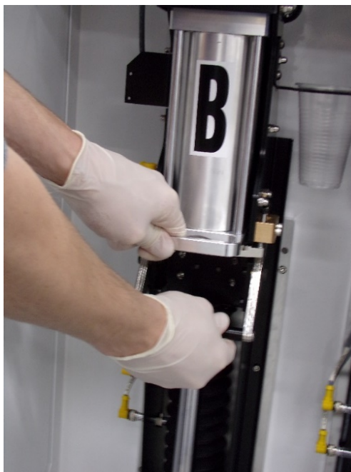
Figure 9: Releasing a Cartridge
