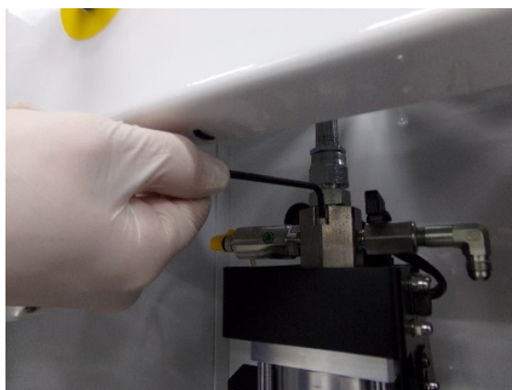
Figure 15: Unscrew Transducer Screws
