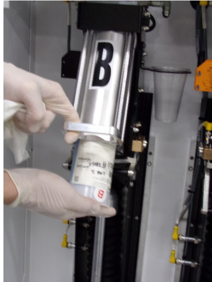
Figure 10: Removing a Cartridge
