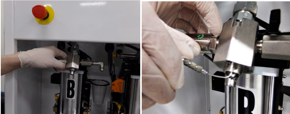
Figure 16: Removing the O-ring
