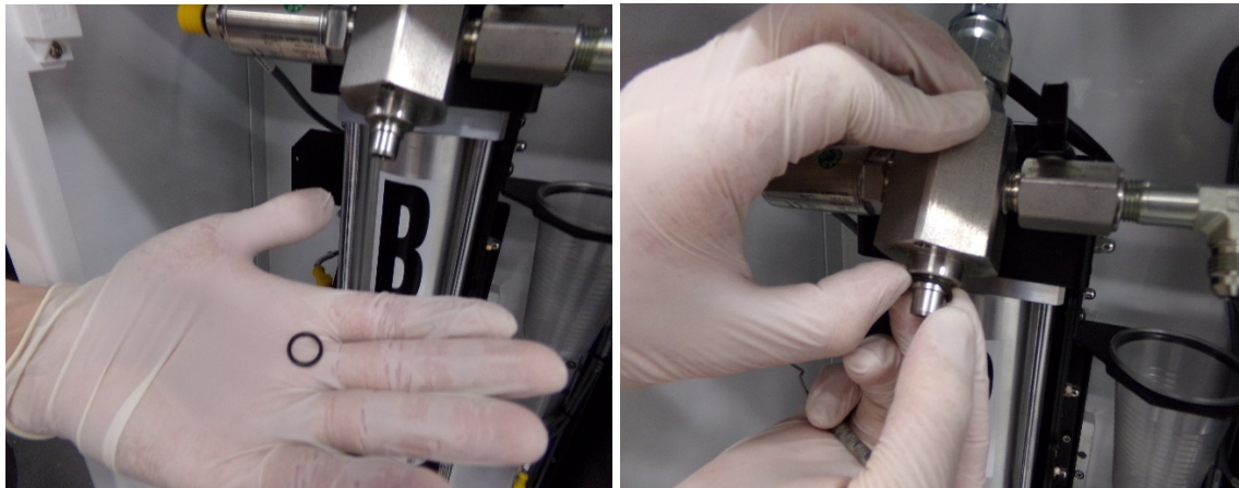
Figure 17: Replacing the O-ring
