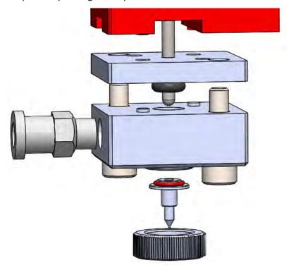
Figure 6: Disassemble the Valve
