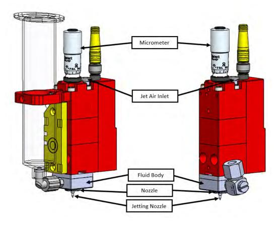
**Figure 1: Pump Components**
