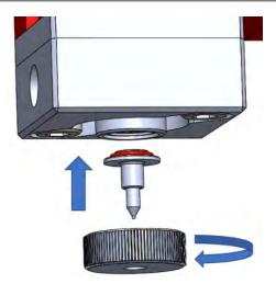
Figure 4: Install the Nozzle
