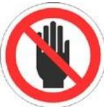
Never put hands or tools in areas with this symbol when the machine is in operation. A dangerous condition may exist.
