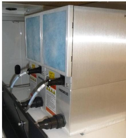
**Figure 34: Connect Lamp Cables**
