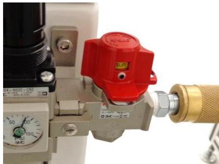
**Figure 10: Example of a Red Air Lockout Valve**
