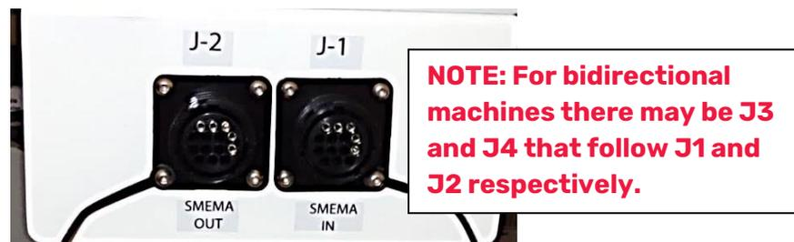
Figure 13: SMEMA Machine Plugs
