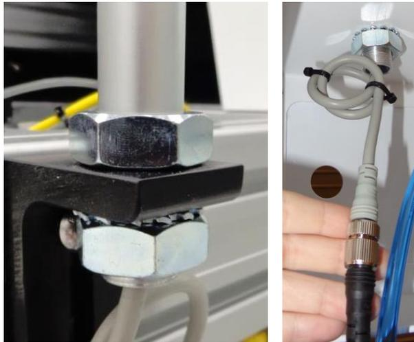
Figure 9: Light Tower Connection
