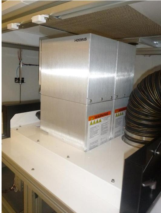
**Figure 33: Install Irradiators**
